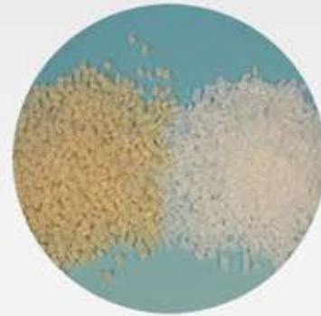
Yellowish color of typical emulsion ABS vs. white natural color of MAGNUM™ ABS.
